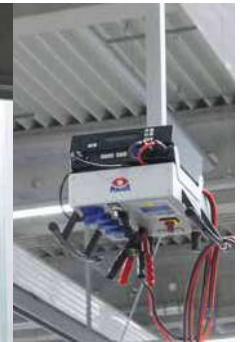
E-BOX version for DEUTRONIK, GYS-FLASH and ELTEK charging computer.
