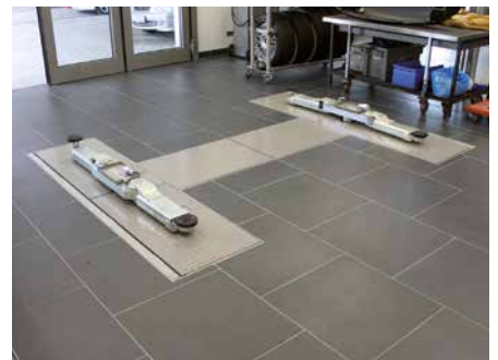
With closed covers, the lift can be used as a standard lift
