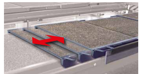
The extended wheel-free jack can be let into the compensating plates continuously.
