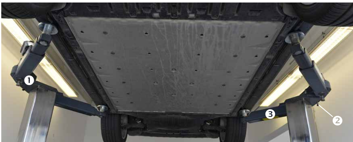
Very flat extension for easy access to car lifting points.
