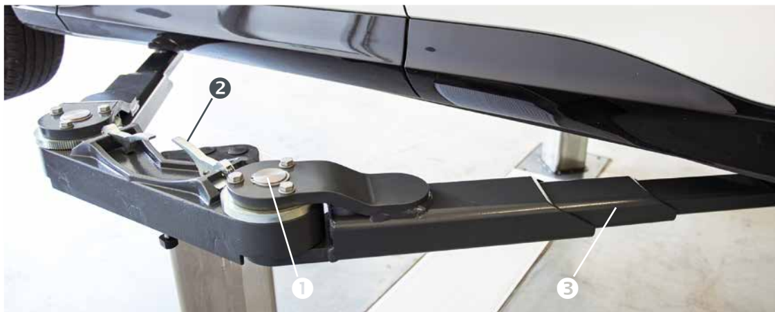
Swing arm support with tool tray.
