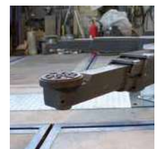
101 mm minimum height of support disc
