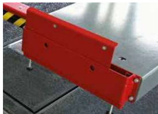
Automatic roll-off protection
