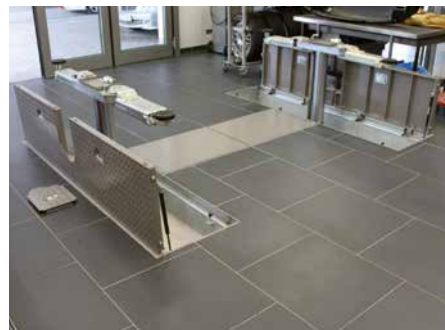
Frame system with cover plate, fully hot-dip galvanised
