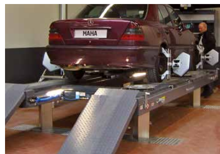
Highly accurate as a wheel alignment lift
