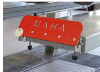
Automatic folding roll-off protection
