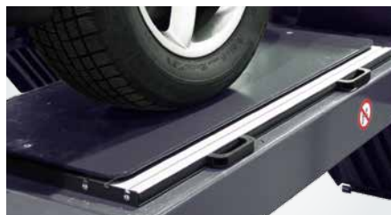
Precision sliding plate Minimal break-off torque of 5 Nm and minimal push force of 15 N, collection grooves for waste water.
