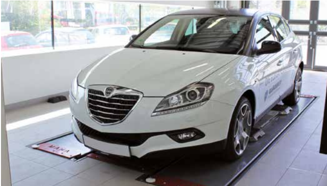
Fully lowered, making it easy to drive on with low ground clearance
