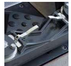
Swing arm support with tool tray.
